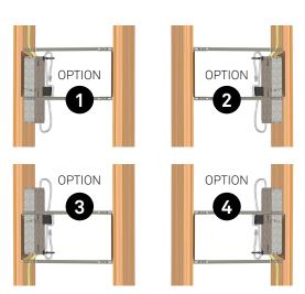
7 Install the two 3-inch (75mm) screws to secure the PSI I
